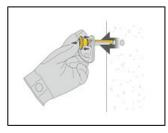
The anchor can be installed and removed for reuse very simply and rapidly, without tools.
