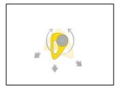
The COEUR hanger can rotate once installed and when laterally loaded during use, allowing it to better align with the systems in place.
